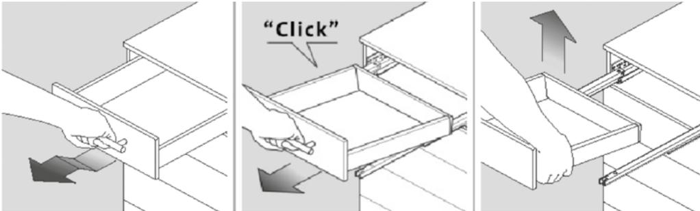
2 SCHUBLADE MONTIEREN ALLE TYPE MODELLE
